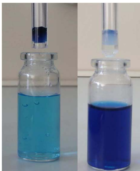
Figure 11. Cryogel samples washed with buffer solution at pH 9.5 (a) and pH 7.1 (b). [Color figure can be viewed in the online issue, which is available at wileyonlinelibrary.com .]
